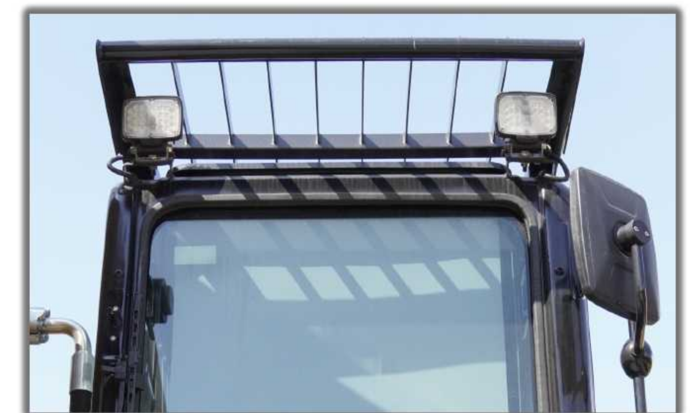
Top protective screening
