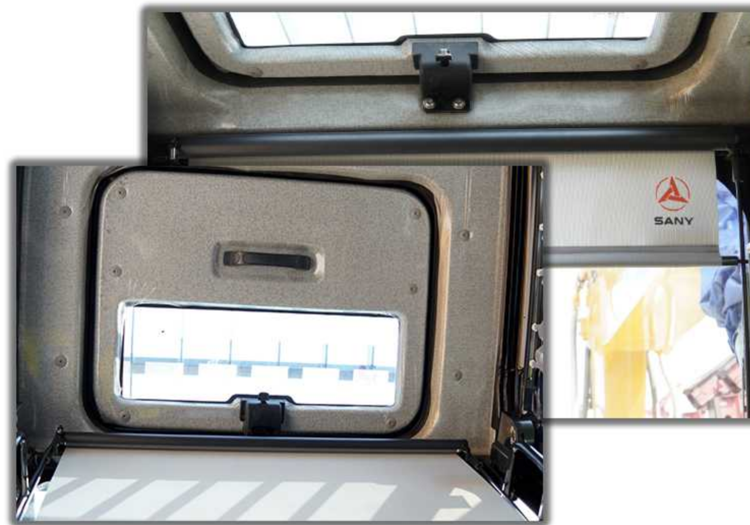
Emergency roof door
